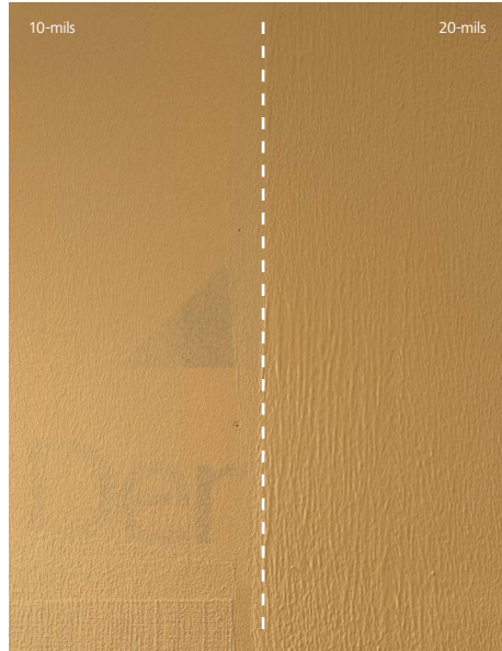
Substrate read-through that is evident at 10-mils WFT (left side) is not apparent at 20-mils WFT (right side).
